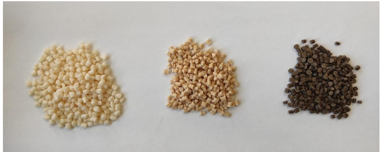
From left to right: First UPM Formi (20% cellulose), second and third samples Smart Materials wood based (pine and coconut respectively).
